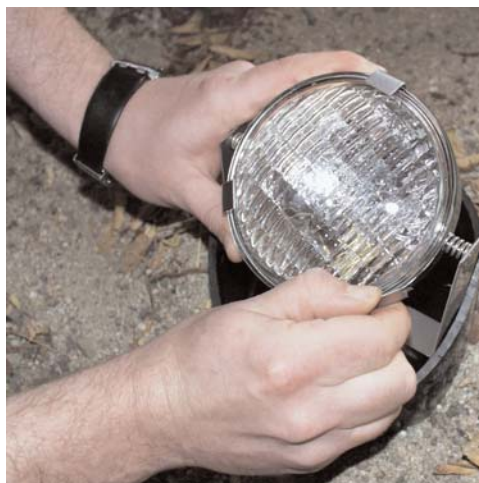
7. Bend metal tabs back into and place to secure lamp to gimbal ring.
