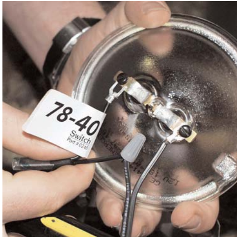
5. Insert new lamp and reconnect screw terminals.
